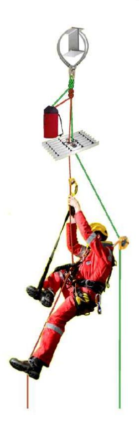
The rescue plan during normal rope access activities as ascending or descending on board under the grating, would be "Rescue from under grating using "Caver lift" technique to switch basic rigging to lowering system.
