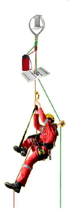
The rescue plan during normal rope access activities as ascending or descending overboard (above water) under the grating, would be "Rescue from under grating using "Caver lift" technique. Switch basic rigging to lowering system and setup cross hauling system through grating, then lower Casualty to Spider Deck.
